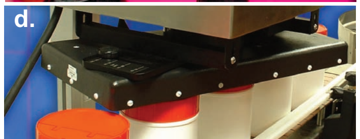
Depending on the cap and container geometry different sealing heads may be required for optimal sealing efficiency. Picture above are common sealing head designs: (a) Tunnel sealing head, (b) Deep tunnel sealing head, (c) Flat sealing head, (d) All-in-one sealing head .
